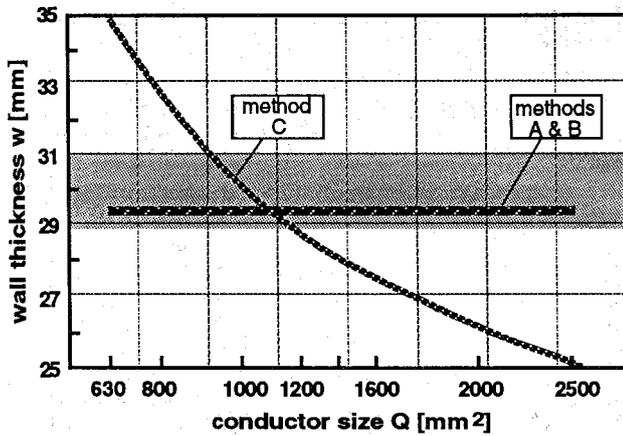
Figure 4: Resulting insulation thickness of 500 kV XLPE cables according to different design methods.
