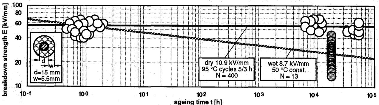
Figure 2: ac voltage ageing tests on 20 kV XLPE cable lengths ( $l = 15$  m). Evaluation by short time ac step tests until breakdown.
