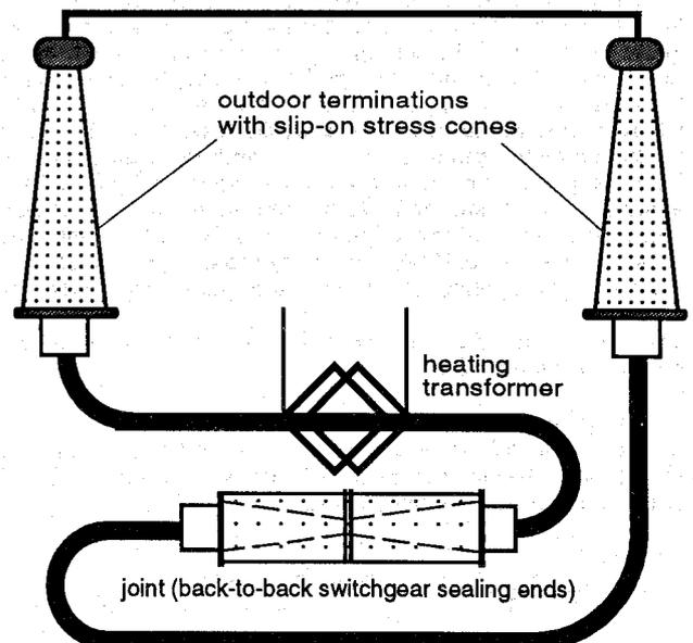
Figure 6: Principle setup for type testing on the 500 kV XLPE cable.
