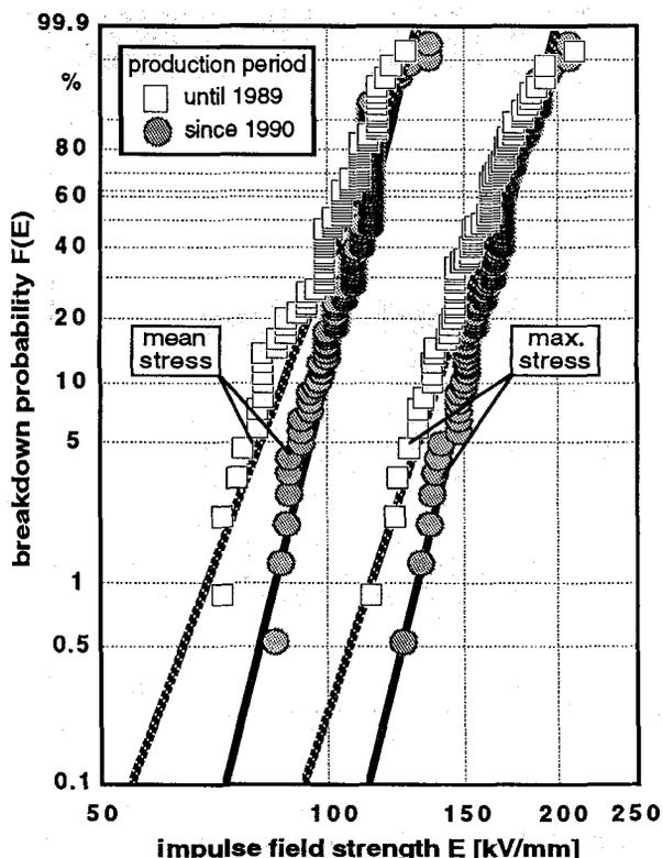
Figure 7: Impulse breakdown strength of HV and EHV XLPE cables from different production periods.
