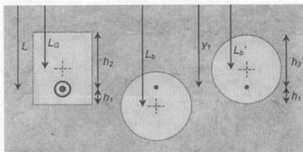
fig.2: Equivalent circular backfills (original and corrected depths)
