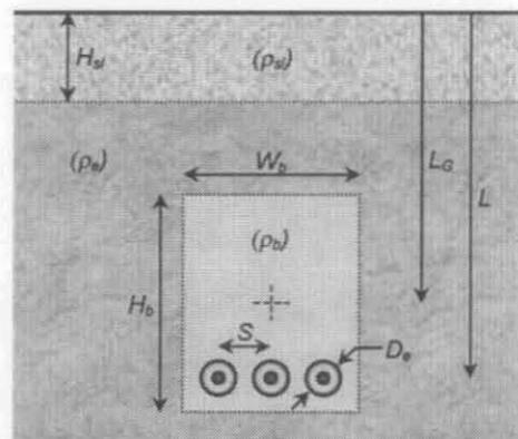
fig.1 : Three cables in a backfill, flat formation
