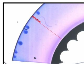
Figure 8: WTs after 7 days in a "homopolymer cable"
