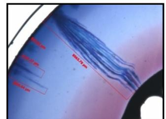
Figure 7: WTs inside the insulation of an aged cable
