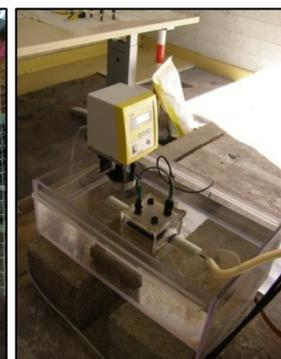
Figure 4: cable sample in salt water during testing
