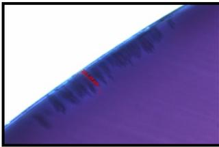
**Figure 9: WTs after 12 days in a "copolymer cable"**
