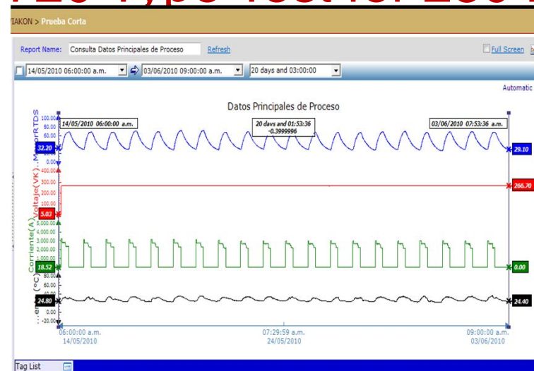
Additional 90 Cycles after IEC PQT @ 105° C & 226 kV
