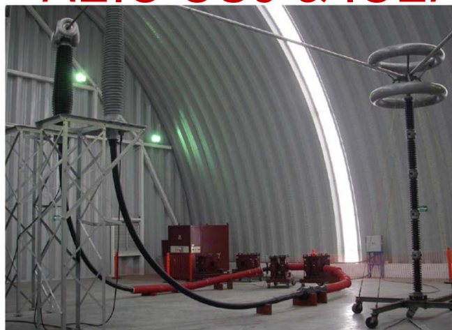
SET UP LOOP – 20 DAYS @ 266 kV IMPULSE TEST \pm 10 @ 1050 kV
