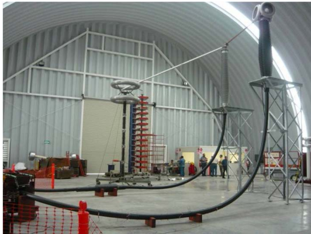
SET UP LOOP – 20 DAYS @ 254 kV IMPULSE TEST \pm 10 @ 1050 kV
