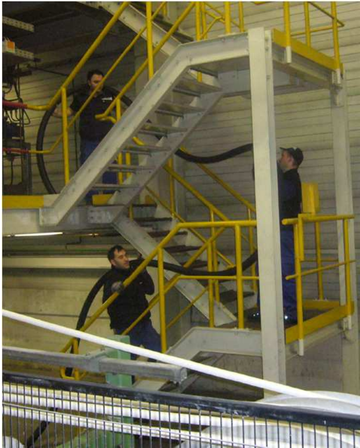
132 kV 1x240 mm 2 Cu Transport to bending test equipment
