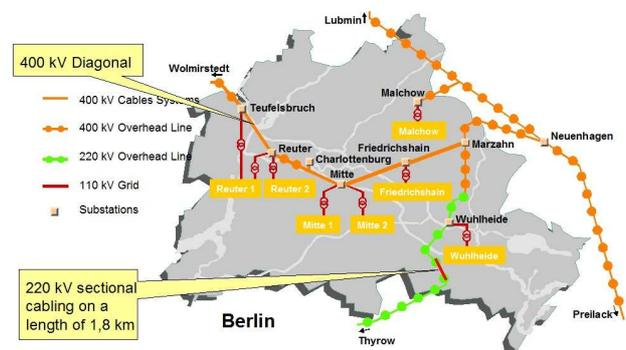
Fig.1: Berlin's 400 kV Diagonal Link
