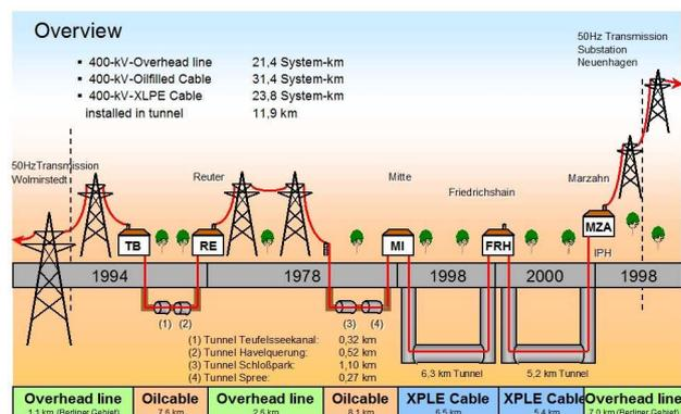
Fig. 2: Overview of 400 kV Diagonal Link
