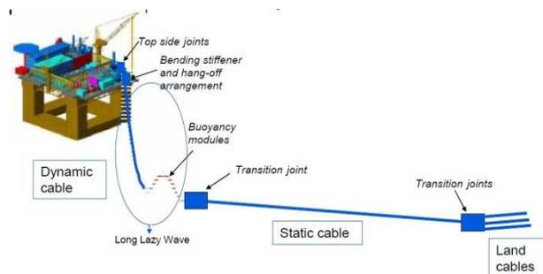
Fig. 1: Conceptual layout of the dynamic cable system.
