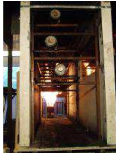
Figure 1: Experimental set-up for fire performance testing of EHV cable
