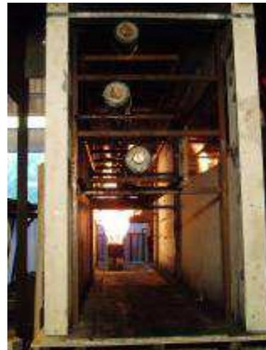
Figure 1: Experimental set-up for fire performance testing of EHV cable
