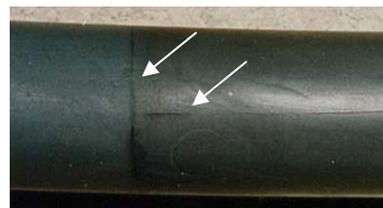
**Figure 1: Knife cuts after removal of the strippable insulation screen was the most common reason of service failure of XLPE cables. This was especially observed for 24 kV cables where the electrical stress is higher than for a 12 kV XLPE cable systems.**
