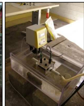
Figure 4: cable sample in salt water during testing
