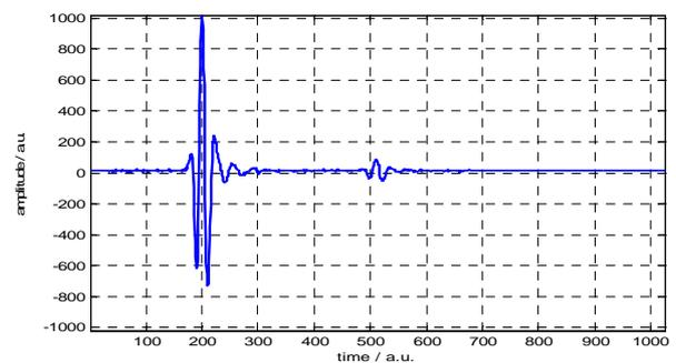
Fig. 1: typical ultrasonic impulse
