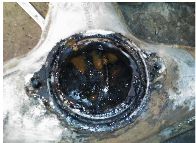
Fig. 2: Water ingress in T-joint
