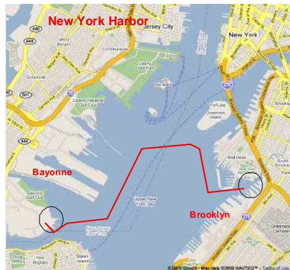
Figure 1. Overview of the 345 kV submarine cable route.
