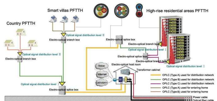
Figure 1: Cabling diagram of OPLC to achieve PFTTH
