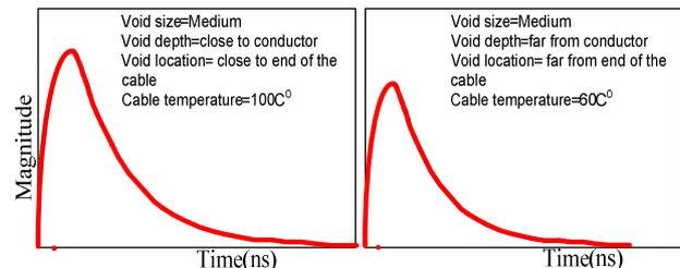
**Figure 1. Two typical PD pulses for two cavities with similar size but under dissimilar conditions.**
