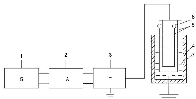
**Fig. 1: Setup used for water trees development: 1- Tektronix CFG 253 voltage generator, 2- Amplifier, 3- High frequency transformer, 4- Ageing cell, 5- Samples, 6- Metal balls to avoid discharges, 7- Water/NaCl solution**
