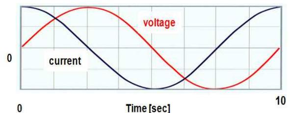
$$\text{Dissipation Factor} = \tan\delta = \frac{\text{true power}}{\text{reactive power}} = \frac{U^2/R}{U^2\omega C} = \frac{1}{\omega CR}$$
