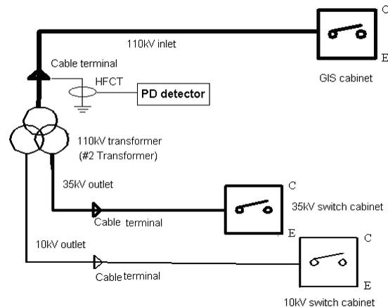
Figure 1. Wiring diagram of the #2 110kV transformer in Huanghoudian transformer substation
