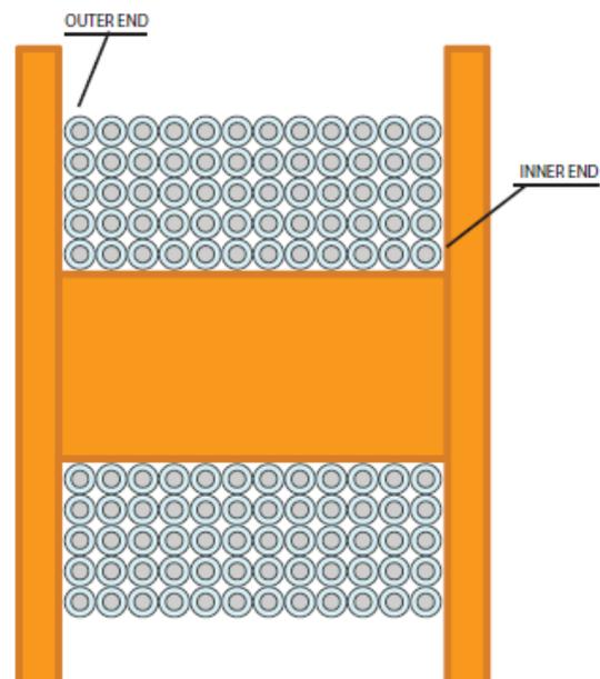
**Figure 1: Schematic description of HV cable on a M30 drum.**
