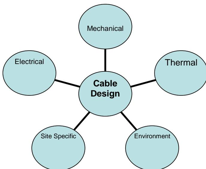
From the engineering point of view, cables are systems whose electrical behaviour is very much dependent upon the materials used within the cable construction. Since a cable system consists essentially of a metallic conductor surrounded by a dielectric, which is in turn wrapped in a metallic screen and protected from the environment, by a non-metallic sheath. The metallic and dielectric materials utilised in the construction thus largely determine its electrical characteristics.
