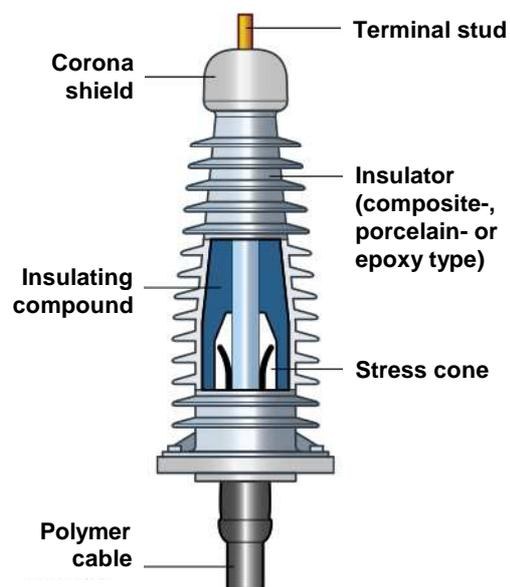
Fig. 1: Design of a termination for polymer cables
