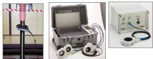
Fig. 1 PD online spot testing equipment, liona
