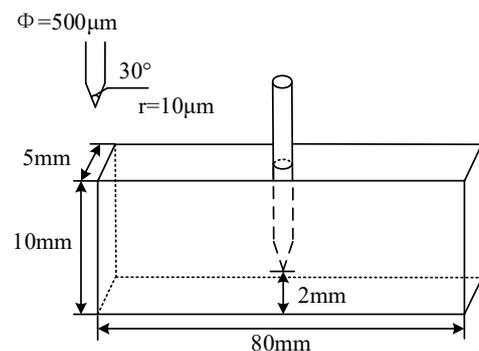
Fig. 1: Configuration of the specimens
