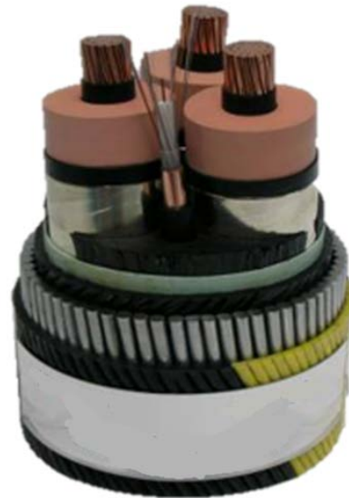
Fig 1: Typical 66 kV submarine array cable with EPR insulation and metal screen made by helically applied copper tapes
