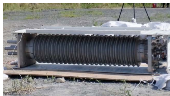
Fig. 1: Sample of durability evaluation of insulators test
