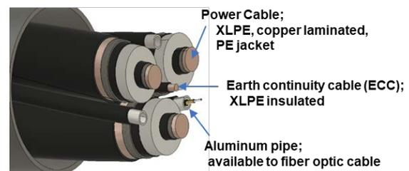
Figure 1: Triplex cable design
