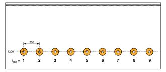
Fig. 1: Example of a circuit with 3 cables per phase
