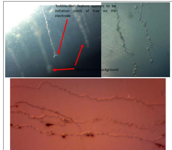
Fig. 3. Electrical treeing observed in joint insulation
