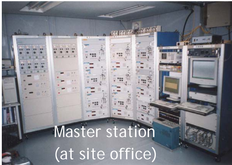
Temporal PD measurement system for whole cable system
