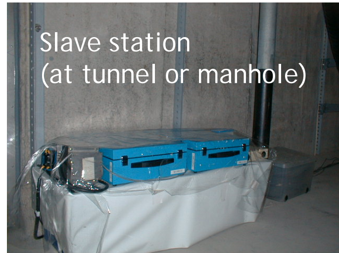
Temporal PD measurement system for whole cable system
