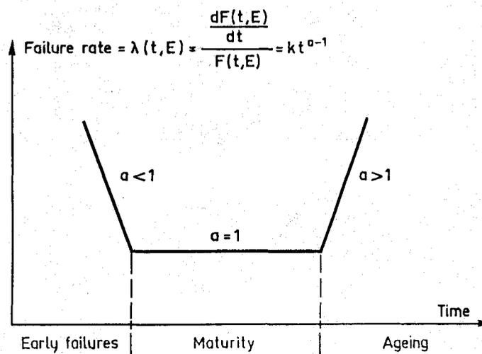
Figure 5c-9. Failure rate as a function of dielectric ageing time.
