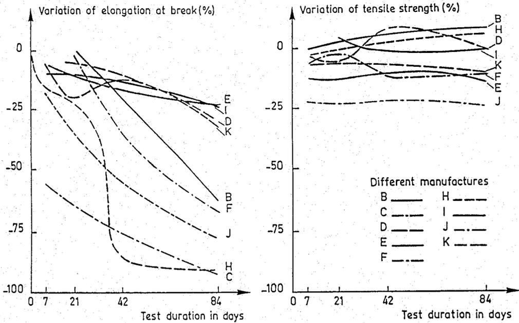
Figure 5c-2. Variation of mechanical properties of XLPE with time at 100°C for a variety of samples from different manufacturers.
