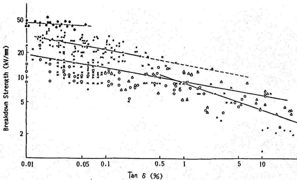
Figure 5e-4. The breakdown strength of XLPE power cables as a function of the loss tangent.
