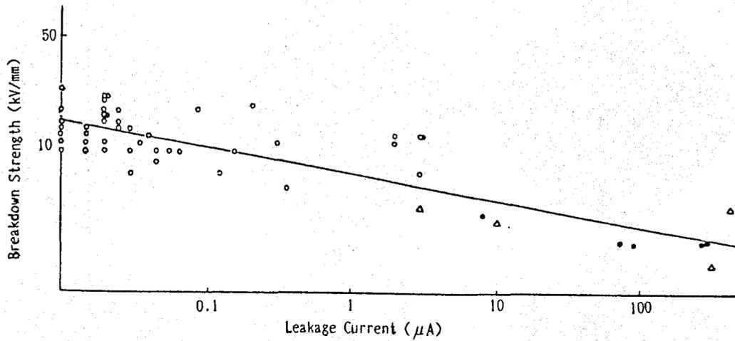
Figure 5e-3. The breakdown strength of XLPE power cables as a function of dc leakage current.
