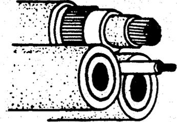
Aluminum conductor cross-section.
