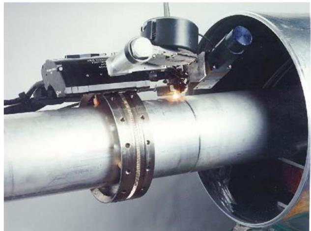
Fig. 2: Orbital welding of the conductor
