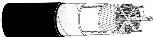
The new cable design should be constituted with the same elements except the neutral conductor which is constituted only with a solid aluminium conductor whose external diameter would be the one of the actual neutral measured on lead.
