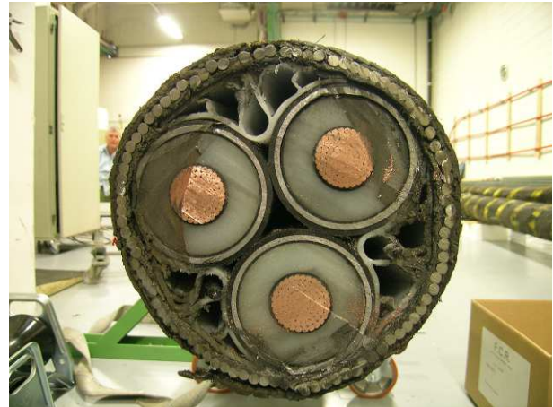
Fig.1: HV cable section before measuring, with lead sheath and optical fibre cables
