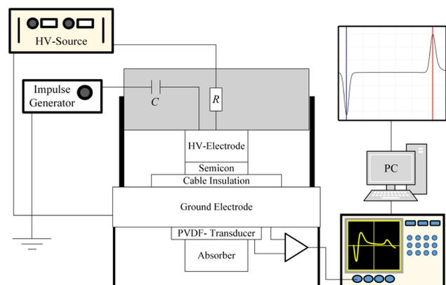
Fig. 1: PEA measurement setup – schematic illustration
