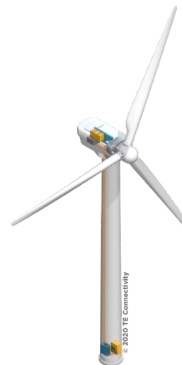
Fig. 1: Typical windturbine with 66 kV cable systems
