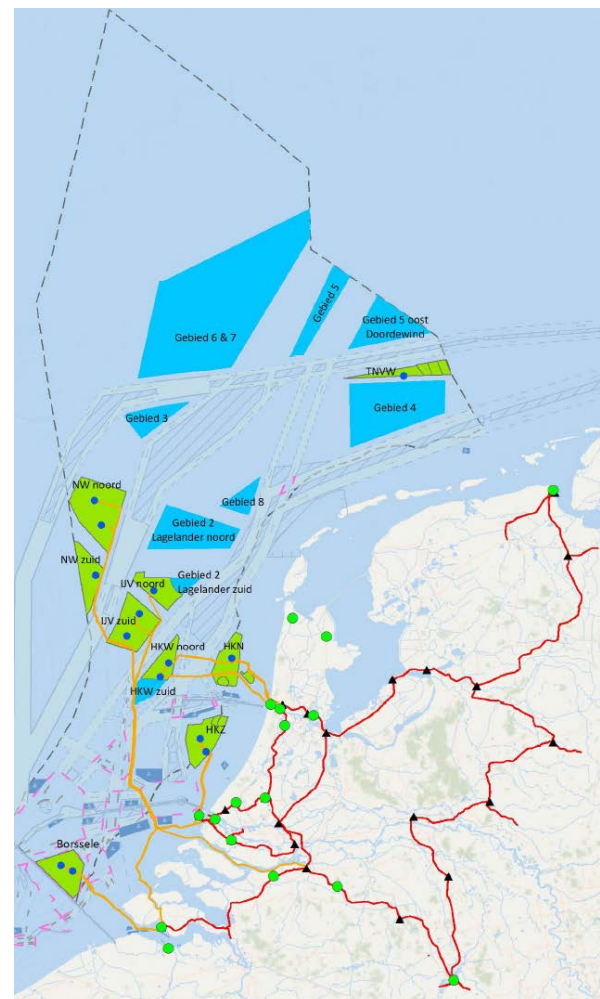
Figure 1 - Cable routes for new wind farm lots (blue) shown of map need to be developed.
