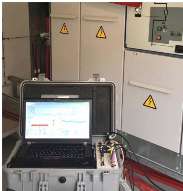
Fig.1: Set up for PD online spot testing
