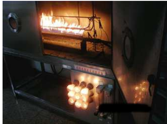
Figure 2: Picture of a small cable sample undergoing fire testing
