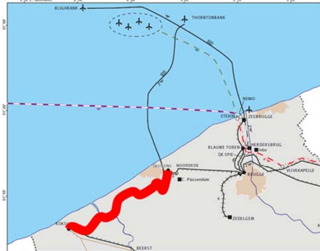
Fig. 2: schema of the coastal region and indication of the 150 kV between Koksijde and Slijkens
