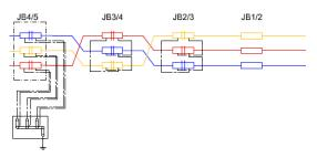
Figure 7 - Cable Direct Cross Bonded 4 cable sections
