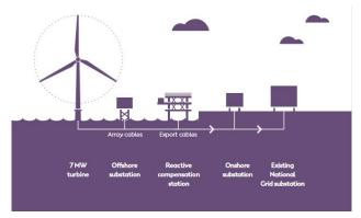
Figure 2 - HOW01 Design Layout
