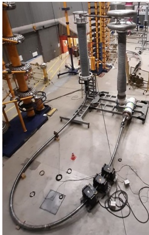
Figure 2: Cable connection assembly test setup for \pm 525 kV Type Test
