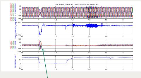
Fault current cleared by AC breaker (3 cycles); full recovery time, from 700 to 1500 ms; with DC breakers or full bridge, time will be less
