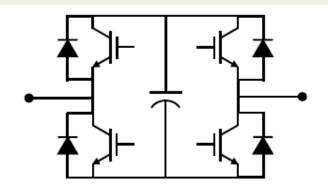
Figure 3 - Full bridge submodule
