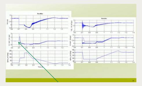
Fault current cleared by Thyristor control in 10 ms; typical straight forward recovery time in the range of 400 ms, including arc deionization
