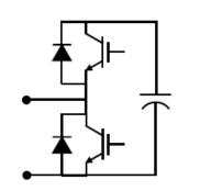
Figure 1 - Half bridge submodule
