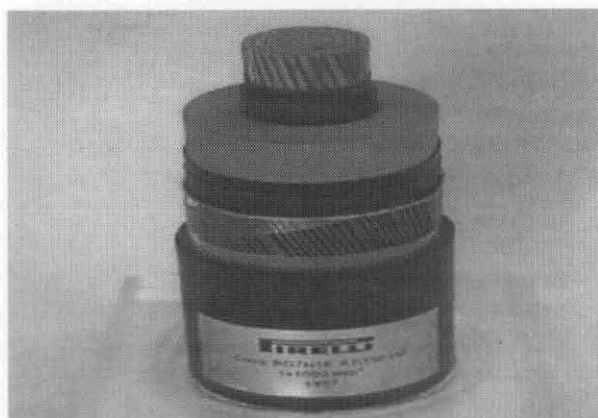
Figure 1 - 150 kV E PR copper wire screen cable with large conductor
