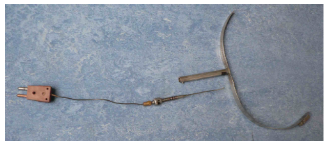
Figure 1 Thermocouple rod (left) and mounting device (right)
