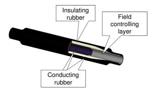
Figure 1. Electrical design of prefabricated joint.
