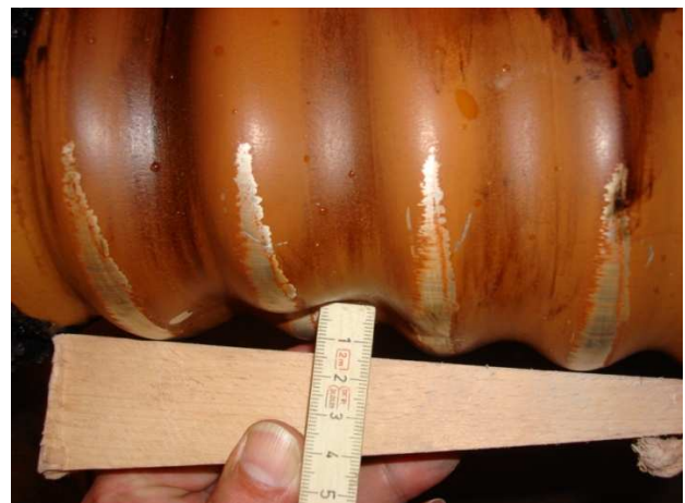
Fig. 3 Corrugated Aluminium Sheath damage after removal of outer polythene sheath
