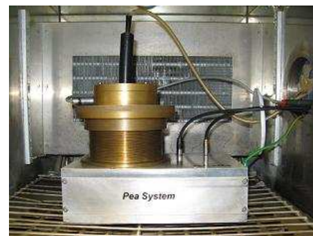
Fig.1: PEA Test bench for plaque specimen up to 30 kV
