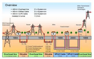
Fig. 2: Overview of 400 kV Diagonal Link
