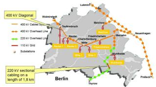
Fig.1: Berlin's 400 kV Diagonal Link
