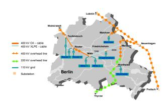
Picture 1: 400 kV diagonal with underlying 110 kV sub-networks.
