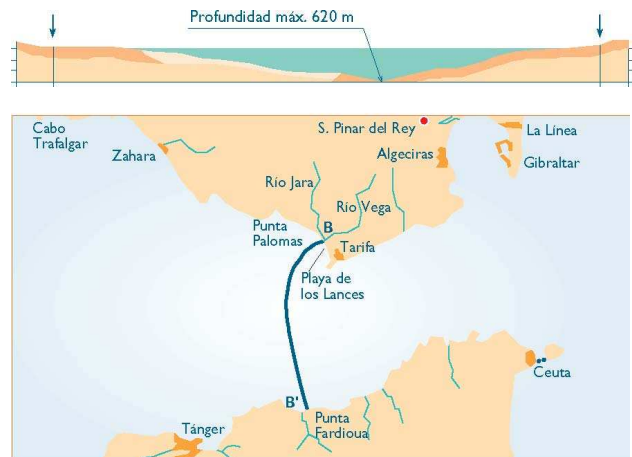
Fig.1: route of the 400 kV Spain-Morocco Interconnection.
